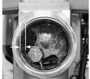
Fig. 4 - Inspect color and amount of grease.
